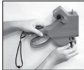
die will lock into shape. The size range is only a guideline and you can use the die that works best for your cable size and shape.
