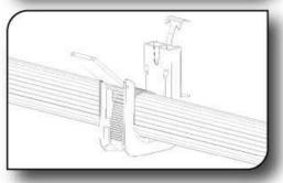
6. Zip Strap can then be secured to hold wires as illustrated.
